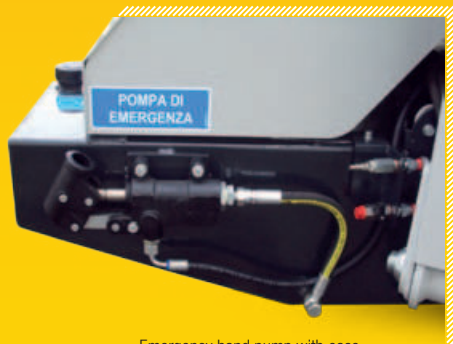
Emergency hand pump with ease of access and operation.
