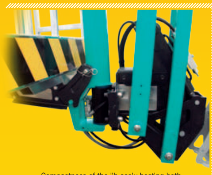
Compactness of the jib ass'y hosting both the load cell and basket rotation system.
