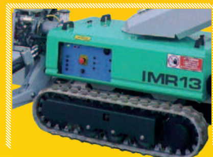
Ground control panel easy to access and protected inside frame guards
