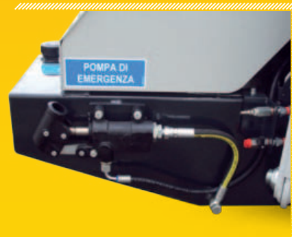
Emergency hand pump with ease of access and operation.
