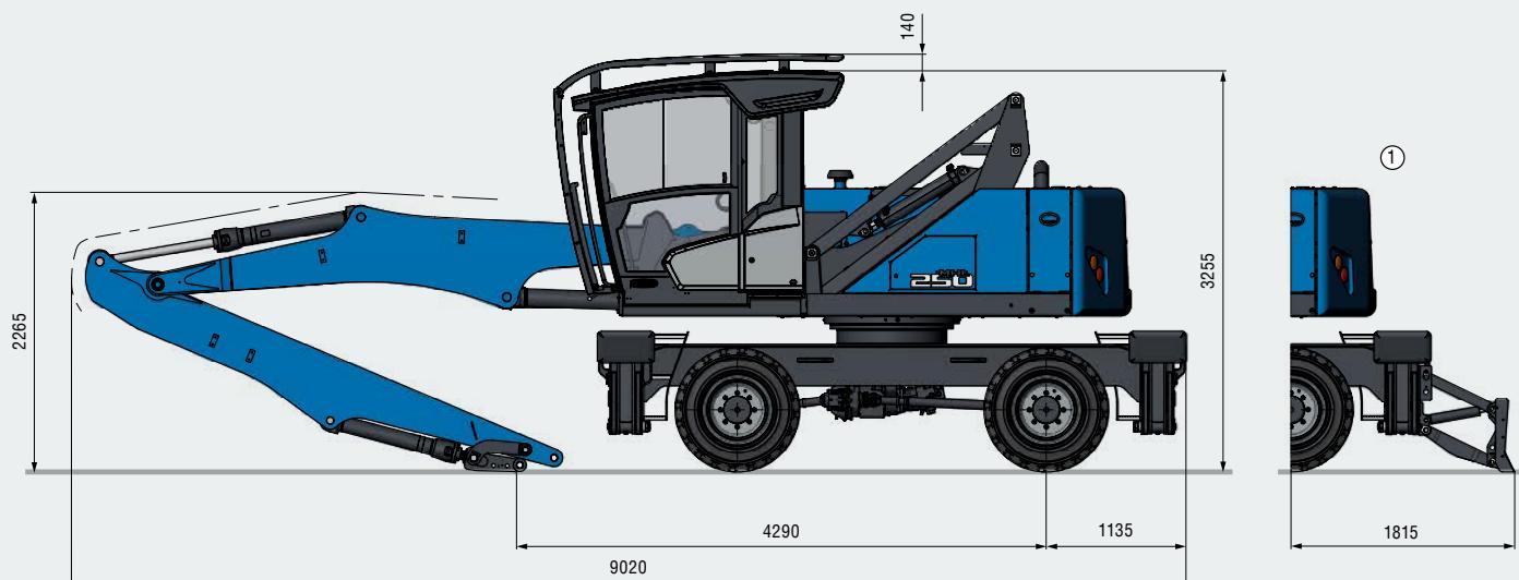
① Transport position with dozer blade; undercarriage rotated by 180°
