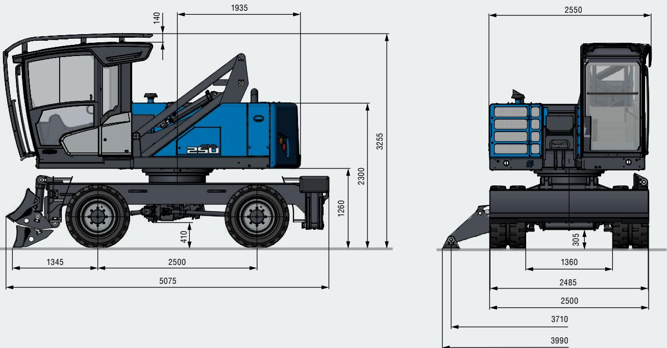
**TRANSPORT DIMENSIONS | TRANSPORTABMESSUNGEN | DIMENSIONS DE TRANSPORT [mm]****DIMENSIONES DE TRANSPORTE | DIMENSIONI DI TRASPORTO | DIMENSÕES DE TRANSPORTE [mm]**
