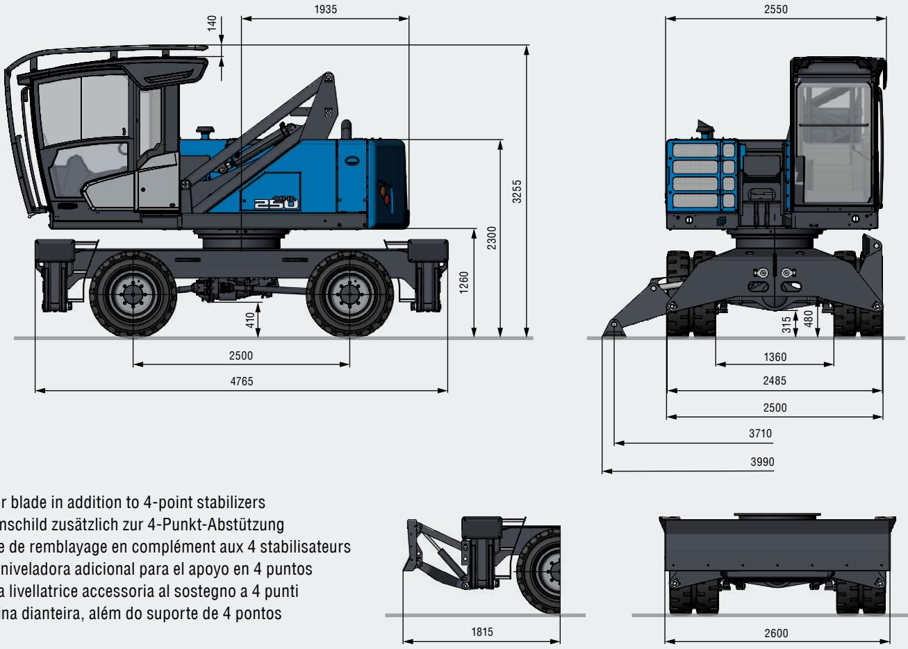
**2-point stabilizers and support blade | 2-Punkt-Abstützung und Stützschild | 2 stabilisateurs et lame d'appui****Apoyo de 2 puntos y placa de apoyo | Sostegno a 2 punti e lama livellatrice di sostegno | Apoio em 2 pontos e placa de apoio**
