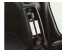
Central fuse box located behind seat
