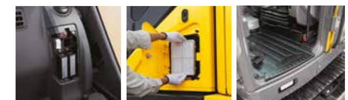
Central fuse box located behind seat Easy-access AC filter Washable cab floor and floor mats
